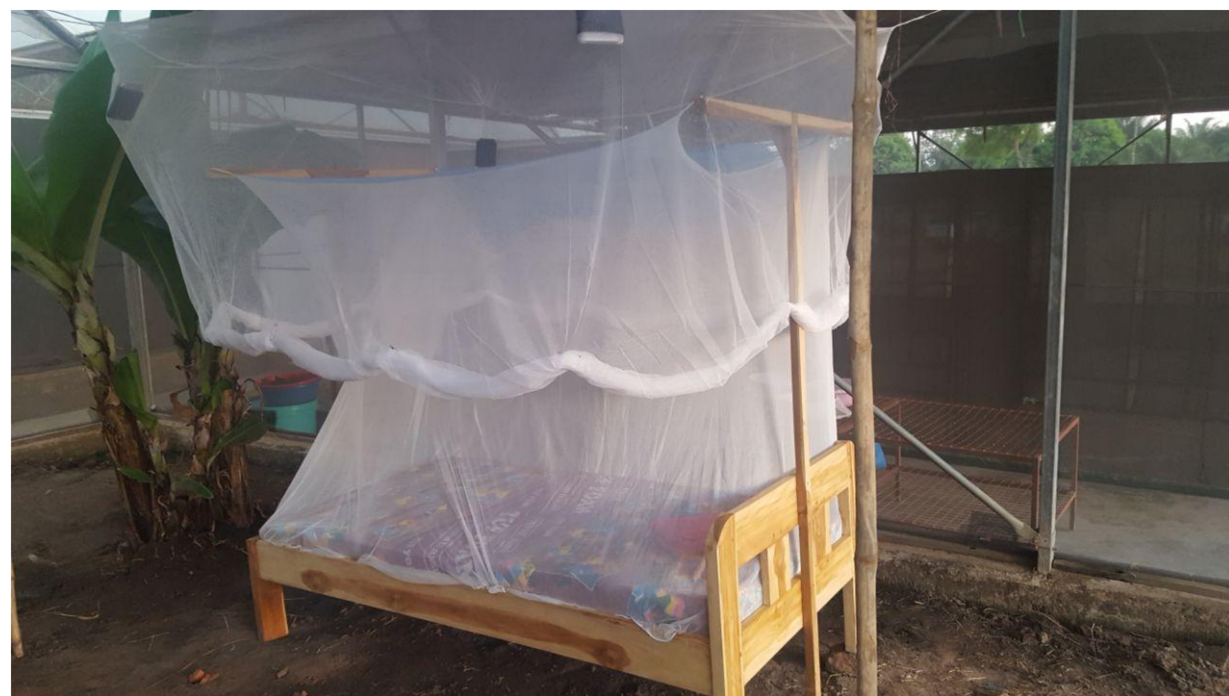
(a) Bednet with four smartphones positioned to trial the best location for recording mosquitoes.
